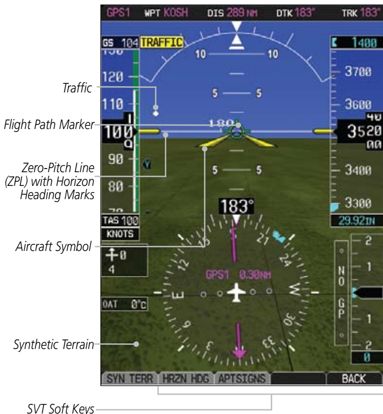
Figure 5-36 SVT on Primary Flight Display
